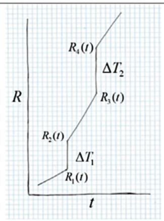
Figure 4: Method for determining the value of temperature coefficient of resistance  $\alpha$ .
