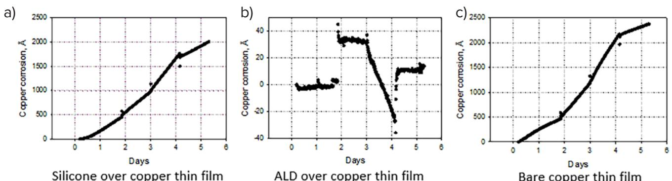
Figure 9: Extent of copper thin film corrosion as a function of time in FoS chamber at 40°C and 15% relative humidity. The nominal thin film temperature was 42°C for 0–1.85 days; 52°C for 1.85–3 days; 64°C for 3–4.16 days and 42°C for 4.16–5.32 days.
