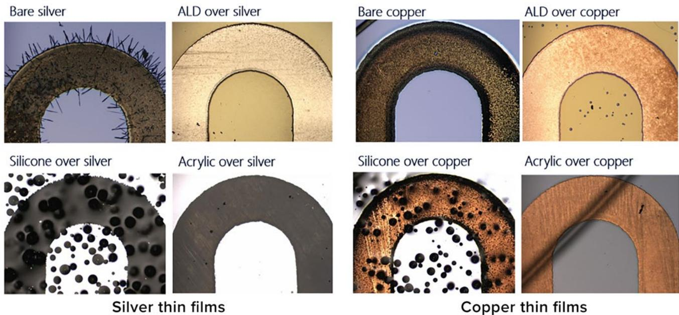
Figure 12: Photographs of serpentine thin films after the 5.32-day test at 50°C and 31% relative humidity.
