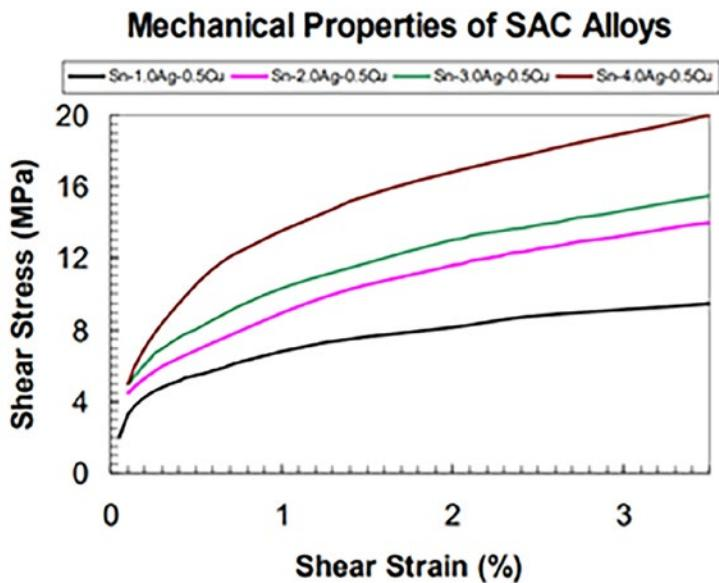
Figure 1: Mechanical properties of SAC alloy.
