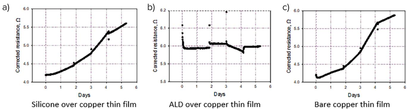
Figure 8: Corrected resistance of copper thin films as a function of time in FoS chamber at 40°C and 15% relative humidity. The nominal thin film temperature was 42°C for 0–1.85 days; 52°C for 1.85–3 days; 64°C for 3–4.16 days and 42°C for 4.16–5.32 days.
