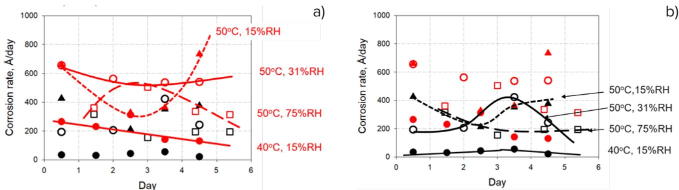
Figure 5: Corrosion rates of a) copper foils and b) silver foils in FoS chamber. Typical time of exposure of foils was one day. Coulometric reduction was used to determine total corrosion product thickness [15].
