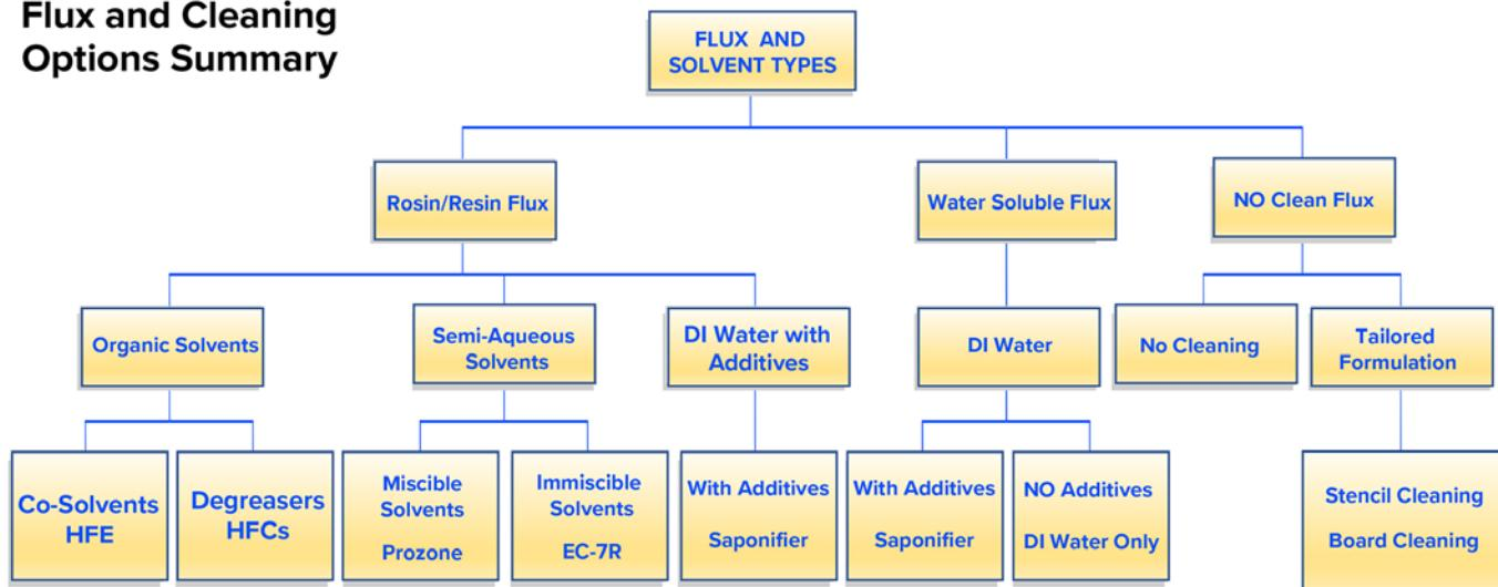
Table 2: Cleaning solvents for different types of fluxes.
