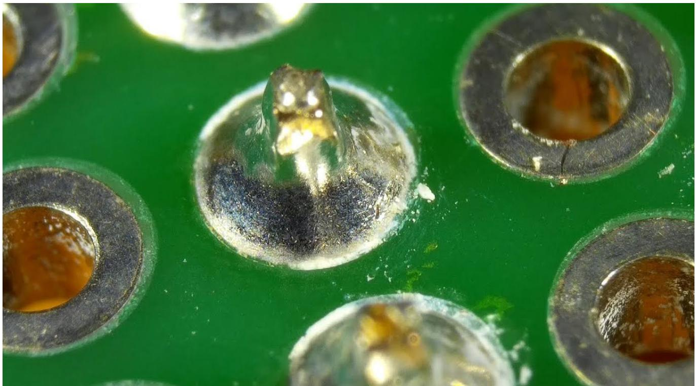
Figure 2: White residue around solder joint.
