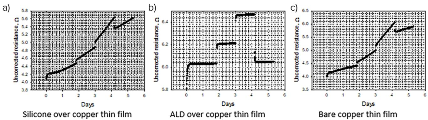
Figure 7: Uncorrected resistance of copper thin films as a function of time at various thin film temperatures in FoS chamber at 40°C and 15% relative humidity. The nominal thin film temperature was 42°C for 0–1.85 days; 52°C for 1.85–3 days; 64°C for 3–4.16 days and 42°C for 4.16–5.32 days.
