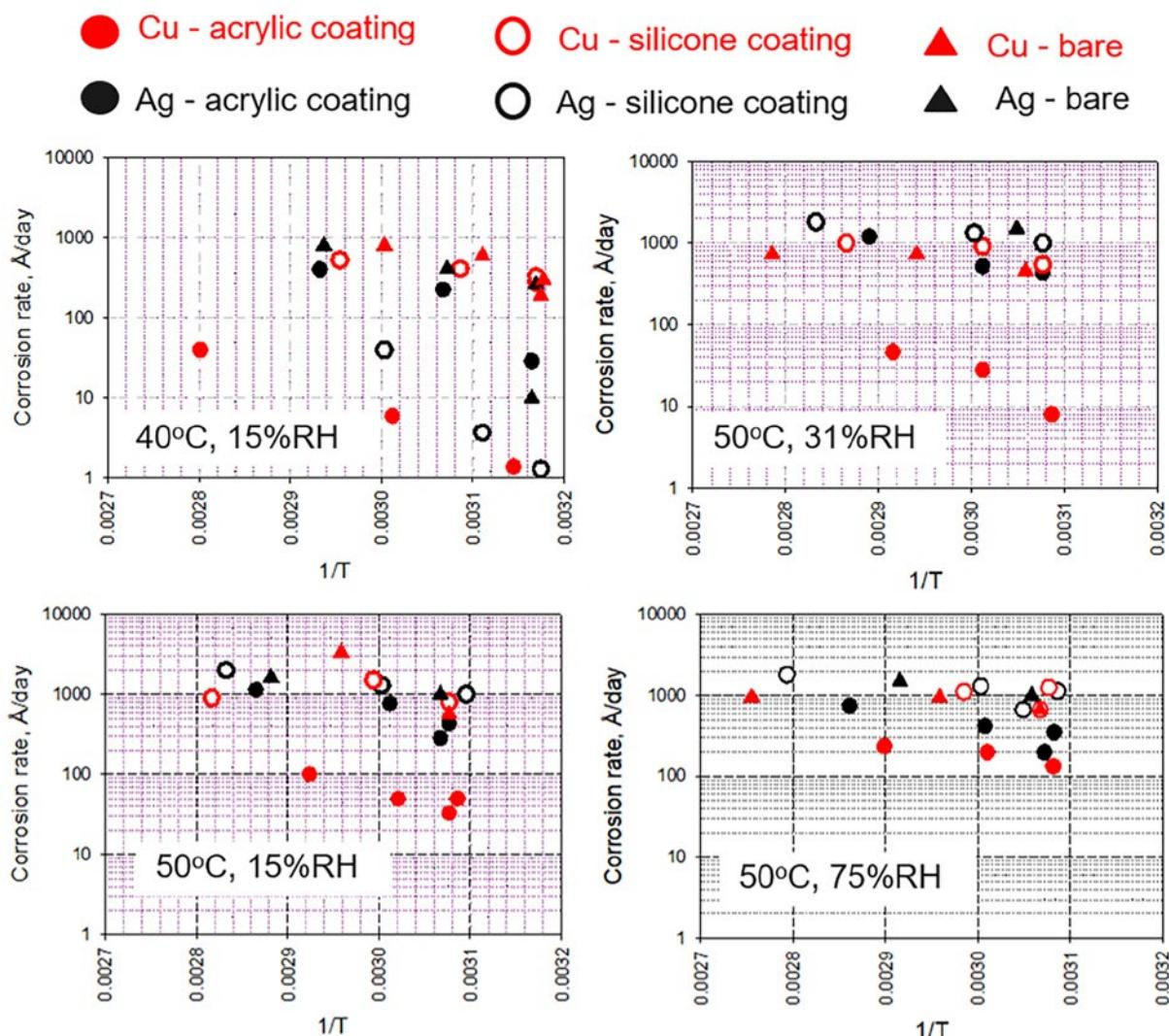
Figure 11: Summary of corrosion rates of bare copper and silver serpentine thin films and thin films coated with acrylic or silicone. ALD-coated thin film corrosion rates are not included in these plots because their corrosion rates were within the limits of the experimental error.
