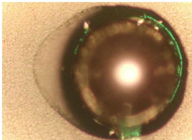
Figure 1: No clean flux residue around through-hole pad.
