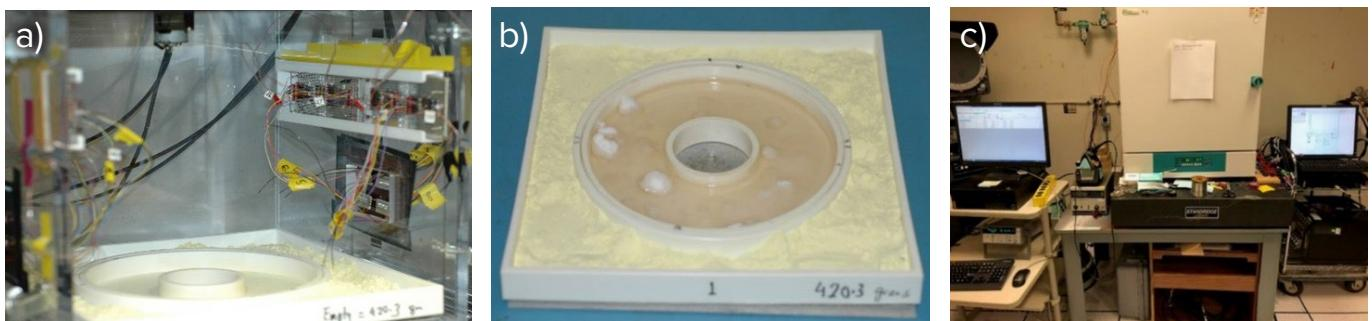
Figure 2: Flowers of sulfur chamber with the thin-film setup: a) Inside view of flowers of the sulfur chamber; b) sulfur and saturated salt trays; c) overall view.
