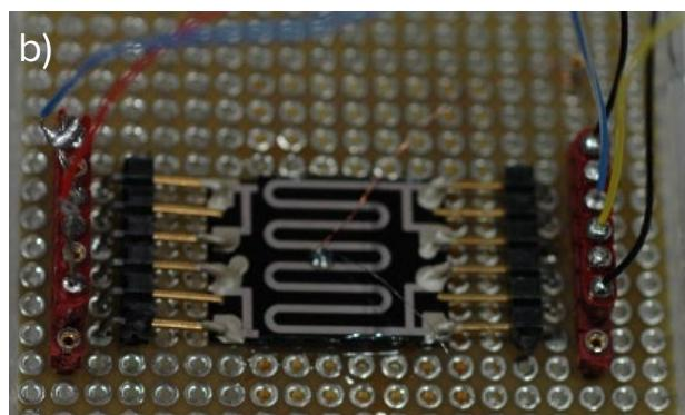
Figure 1: a) Serpentine thin-film setup. In earlier works the bottom thin films were to heat the top film; b) In this work the bottom films were not used.
